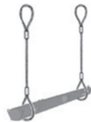
"Bilancino" (1 truss beam + 2 suspension points)
